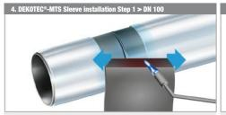
Warm the adhesive side of the sleeve on the side with the 45° chamfer to a length of approx, 200 mm (8").
