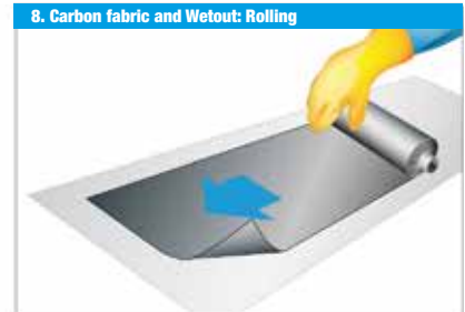
8. Carbon fabric and Wetout: Rolling
