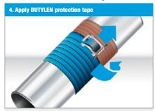
Apply the BUTYLEN-AS50 (VivaxCoat®-LT/-MT) or BUTYLEN-ET100 (VivaxCoat®-HT) mechanical protection tape on top of the anti-corrosion tape, with a cover rate of 50% (1x50% of covering for the HR class). The mechanical protection tape must fully cover the anti-corrosion protection tape and exceed at least 5cm. For effective implementation, it is recommended to use a DEKOMAT® coating machine.
